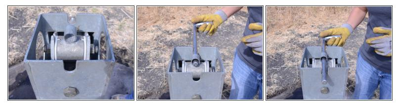
• Insert the T-handle into the top cylinder of the exposed pump rod.
