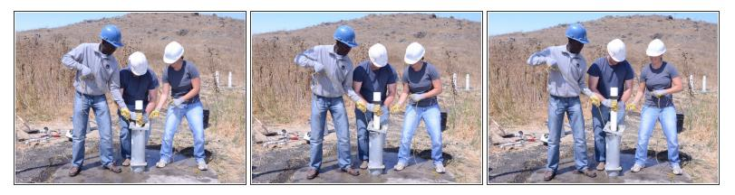
• Lift the casing from the borehole, simultaneously pulling up on the ropes to support the casing.
