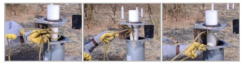
• Untie knots from the flange, holding on to the loose ends of the rope.
