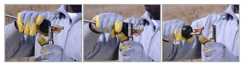
Unhook the first connection by pushing it out and down, then pulling it away from the rest of the rod.
