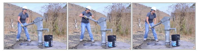
• Perform a water test on the pump, by raising and lowering the handle a full 40 strokes. A properly performing pump will yield greater than 10 liters.
