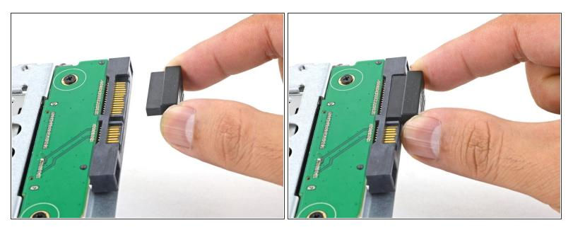
• Plug the included sensor-enabled SATA power cable into the enclosure's port.
