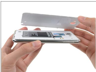
Lift and remove the rear case from the phone.
