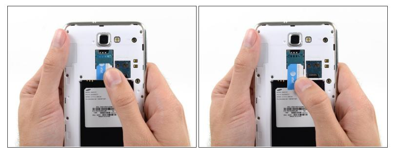
• Slide the SIM card out the rest of the way with your thumb and remove it from the device.
