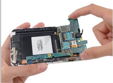
Remove the motherboard assembly from the display assembly.
