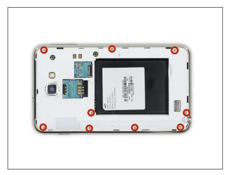
Remove the nine 3.4 mm Phillips #00 screws securing the midframe to the display assembly.
