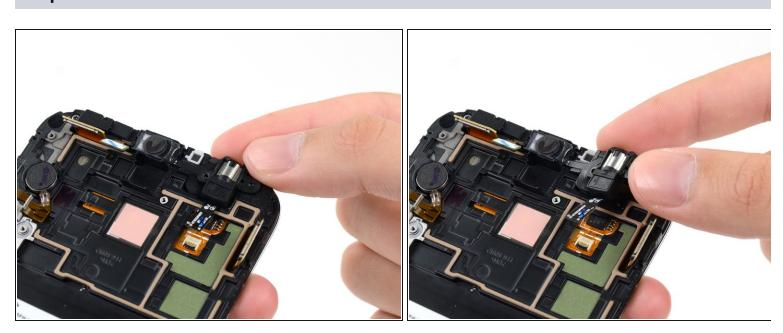
Grasp the headphone jack portion of the assembly and lift it out of its groove in the display assembly.
