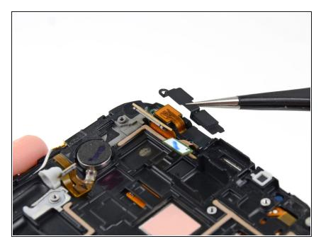
Remove the front-facing camera bracket.
