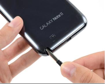
Grasp the end of the stylus and remove it from its slot in the midframe.
