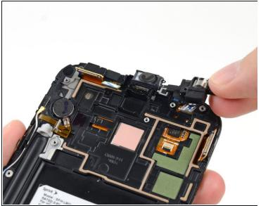
Gently pull the headphone jack straight up without twisting the cable to remove the earpiece speaker portion from its recess.
