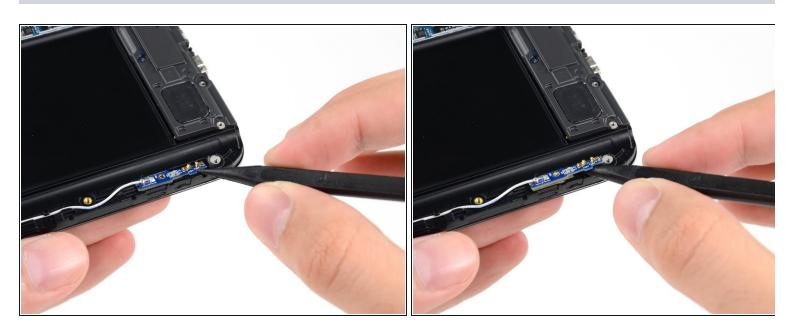
• Insert the tip of a spudger under the antenna board to free it from the adhesive holding it to the display assembly.
