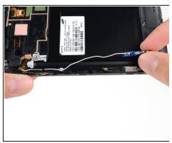
• Gently de-route the antenna cable from its channel in the display assembly.
