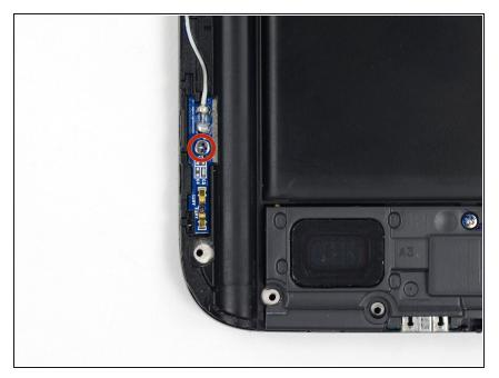
Remove the 3 mm Phillips #00 screw securing the antenna board to the display assembly.
