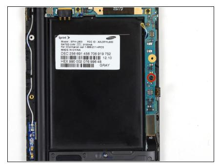
Remove the 3 mm Phillips #00 screw securing the motherboard to the display assembly.
