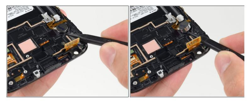
Insert the tip of a spudger under the vibrator to free it from the adhesive holding it to the display assembly.
