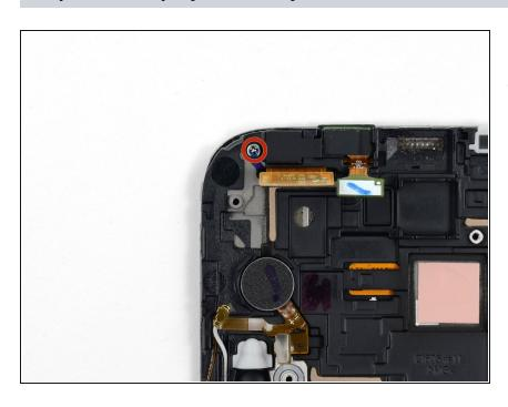
Remove the 3mm Phillips #00 screw from the front-facing camera bracket.
