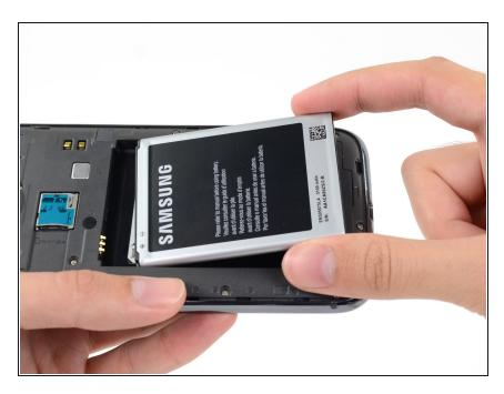
Remove the battery from the midframe.
