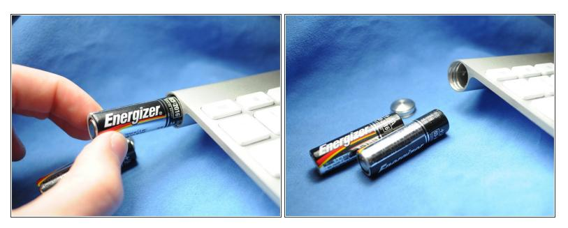
• Slide the two (three on the previous generation) replacement AA batteries into the battery compartment. Verify the positive and negative terminals are facing the correct orientation.
