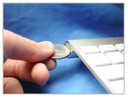
• Use a coin to remove the battery compartment cover.
