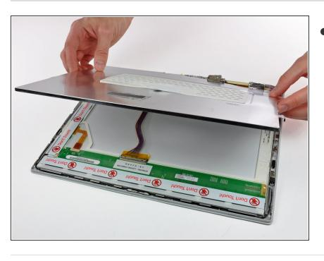
Lift the thin steel LCD cover off the LCD.
