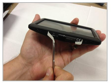
Peel back the sticker on the bottom of the device to reveal the two screws.
