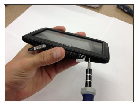
• Unscrew the two T5 Torx screws.
