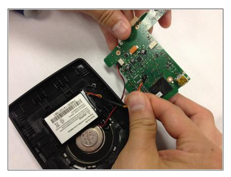
• Remove the motherboard from the back plate.
