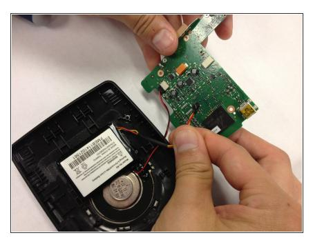
Plug the new battery into the white receptacle on the green motherboard.
