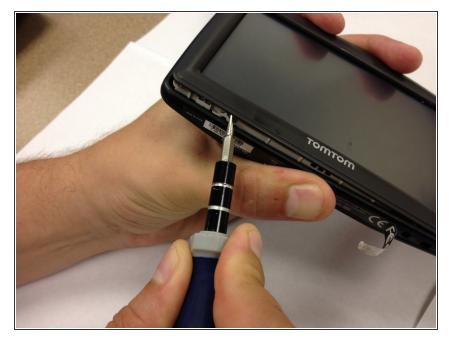
Wedge the flat head of the screwdriver into the edge of the device. Gently lift the screen from the cover.
