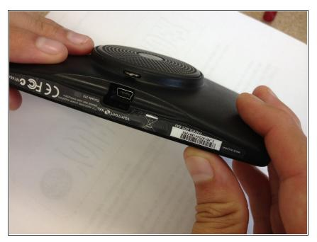
Reconnect the yellow ribbon cable and connect the screen and back plate back together.
