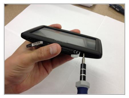
Insert the t-5 screws and tighten to secure.
