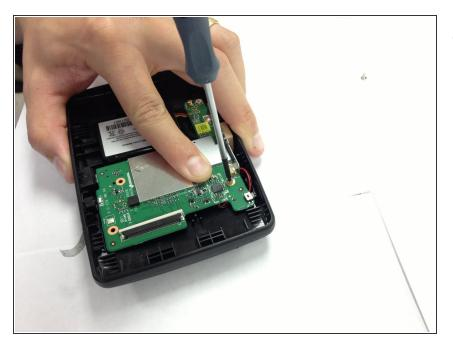
Transfer the green motherboard back into the back plate and secure it with the 3 screws.
