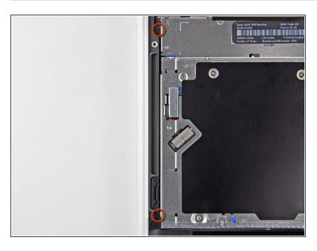
Remove the two 2.5 mm Phillips screws securing the optical drive to the upper case near the optical drive opening.
