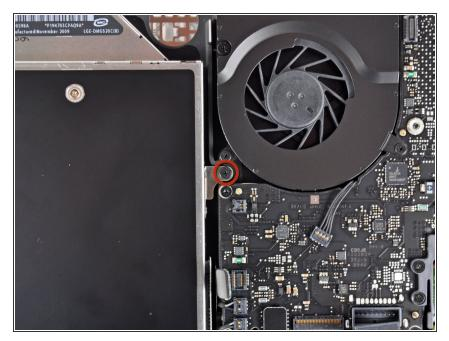
Remove the single 4.5 mm Phillips screw securing the optical drive bracket to the upper case near the fan.
