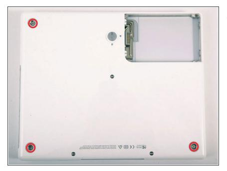
• Remove the three newly-revealed Phillips screws.
