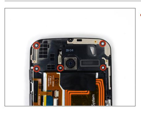
Remove the five 3 mm T3 Torx screws from the headphone jack/speaker assembly.
