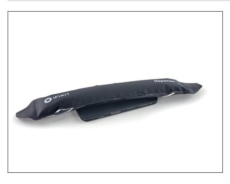
Heat an iOpener and lay it over the phone for approximately 90 seconds to loosen the adhesive securing the back cover.
