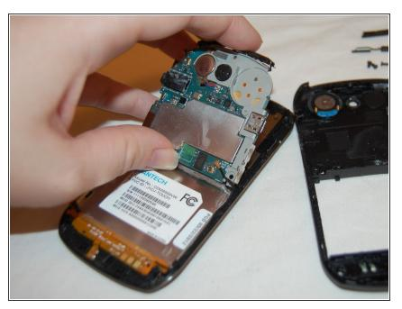
• Loosen the motherboard from the front case.
