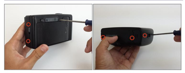
• Use the screwdriver to unscrew the indicated screws from the left, right, bottom, and back sides of the camera.
