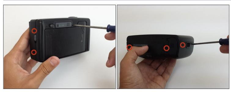
• Use the screwdriver to unscrew the indicated screws from the left, right, bottom, and back sides of the camera.
