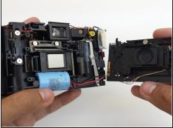
• After removing the metal clip in the previous step, the front face plate can be removed.
