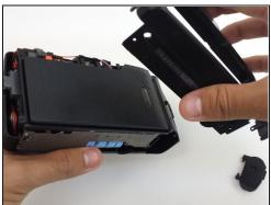
Loosen the back cover from both the left and the right sides of the camera.
