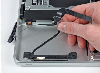
Carefully peel the hard drive and IR sensor cable off the right speaker body/upper case and remove them from your computer.
