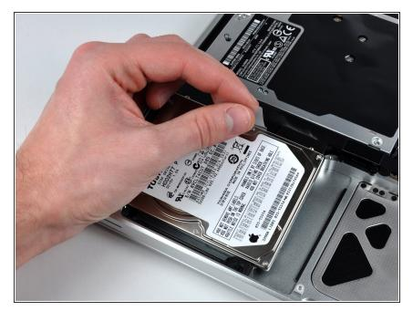
Lift the hard drive by its pull tab and pull it out of the chassis, minding the cable attaching it to the computer.
