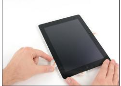
• Slide the opening pick along the left edge of the iPad, releasing the adhesive as you go. The adhesive is thin here due to the digitizer along the whole left side. Make sure the pick is not too deep (max 1/2 inch) 10 mm to prevent damaging the digitizer.
