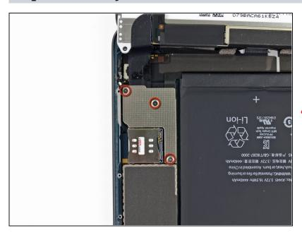
Remove the three 1.3 mm Phillips #00 screws securing the connector shield to the logic board.
