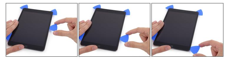
• Continue to slide the pick down the right edge of the iPad, releasing the adhesive.
