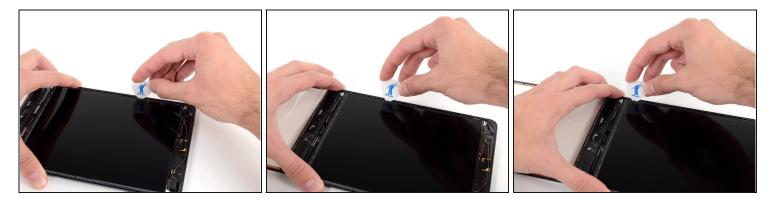
• Insert the guitar pick into three more locations down the left side of the LCD and bend it over in each location, to slide the LCD over to the right side of the rear case.
