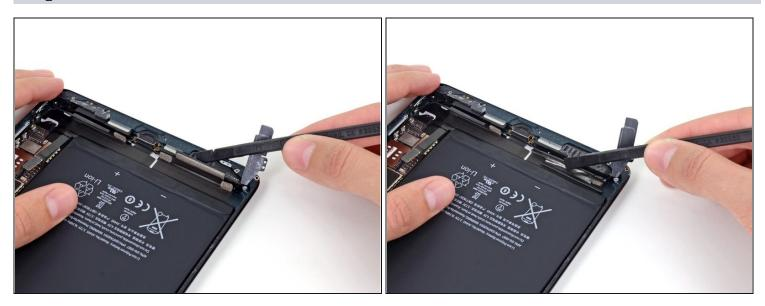
• Use the flat end of a spudger to fold the left-hand wide piece of tape away from the left speaker.
