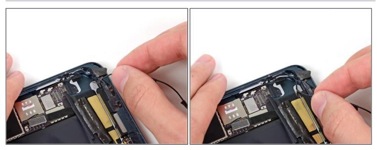
• Pull the antenna cable away from its recess in the rear case.
