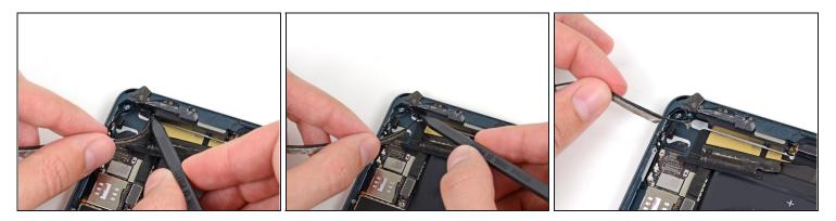
• Use the tip of a spudger to remove the small piece of tape securing the antenna cable in the bottom right corner of the iPad.
