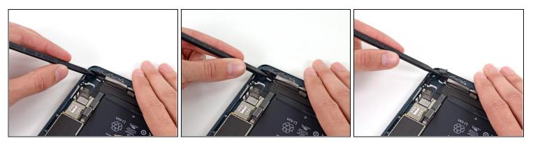
• With the tip of a spudger, peel up the larger piece of tape covering both antenna cables near the bottom of the rear case.
