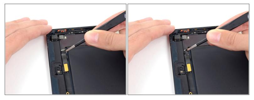
Use a pair of tweezers to peel up and remove the small piece of tape covering the front-facing camera cable connector.
