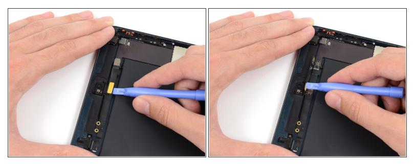
Gently fold the front-facing camera cable upwards (roughly at a 90-degree angle), exposing the bottom side of it.
