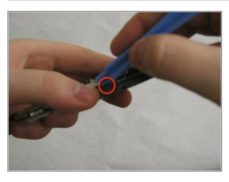
Use a pick or other small tool to pop the small plastic clip holding the LCD panel on
