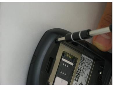
Use a T6 Torx screwdriver to remove the 6 screws holding the rear of the phone.
