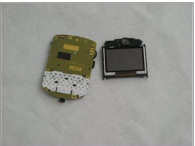
Pull the LCD screen off of the board.
