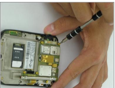
Remove the indicated screws using a T6 Torx screwdriver.
