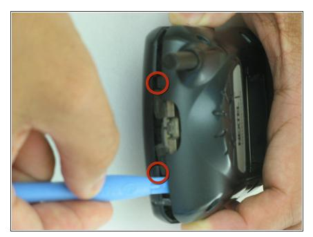
Repeat the process of unlatching the clips for the top section of the Blackberry.
