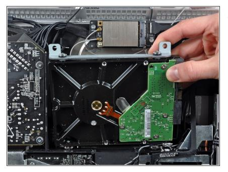
Slightly rotate the hard drive out of the outer case and lift it up off its mounting pins toward the top edge of the iMac.
