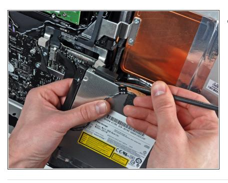
Use the flat end of a spudger to help disconnect the optical drive cable.
