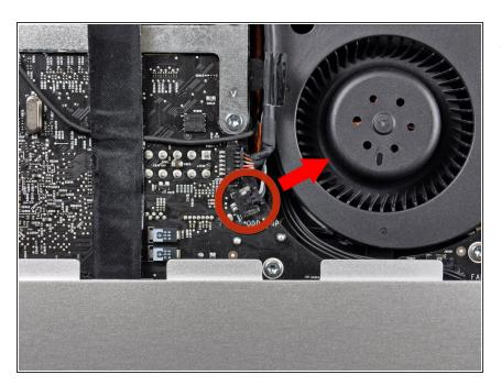
Pull the optical drive thermal sensor connector straight away from its socket on the logic board.
