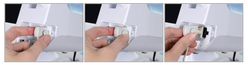
Depress the spring tab on the temperature probe cable connector and withdraw it from the probe port.
