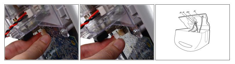
• Disconnect the communications power cable from its socket (labeled J50 in the service manual).
