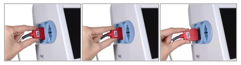
• Place your thumb and forefinger on the Pulse oximetry (SpO2 or combined SpO2/SpHb) cable connector. Squeeze the side tabs until the connector releases.
