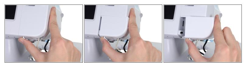
• Remove the cover of the temperature module by pressing the tab and sliding the cover to the right.
