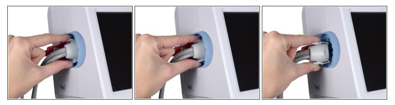
• Place your thumb and forefinger on the blood pressure (NIBP) hose connector. Squeeze the side tabs until the connector releases.
