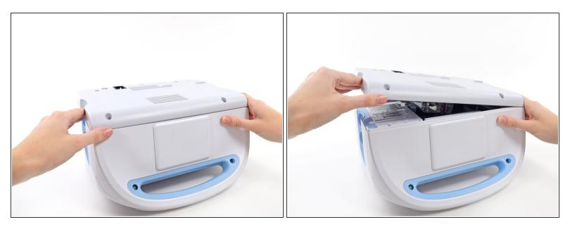
With the handle/alert bar facing you, begin to lift the rear housing from the left side, holding the right side securely.
