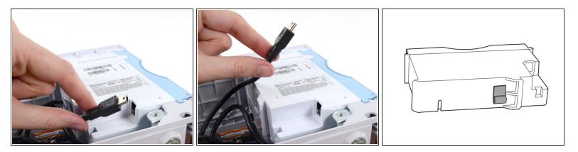
• Remove the USB cable from the retaining clip on the module.
