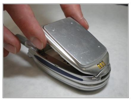
Remove the battery by lifting up and rotating the battery away from the bottom edge.
