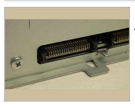
The connector system used for the front panel has blades instead of pins, and seems to be robust.
