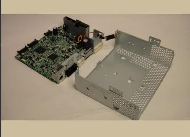
The bottom cover is separated from the main PCA by removing the 5 screws seen in the top view.
