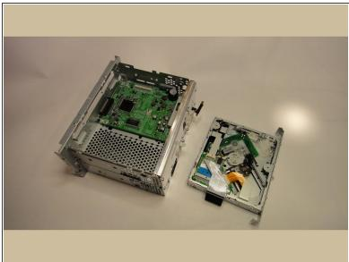
Lift the CD drive out of the unit, starting at the rear.
