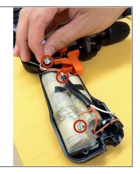
Reconnect the battery wires to the battery terminals by fitting the wire terminals over the battery terminals where they were originally fitted.
