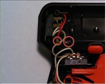
Use the pliers to "slide" the wide sides of the motor terminals to firmly secure the wires back to the terminals.
