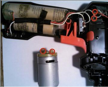
• Pull out the motor and lay it next to the drill; keep in mind that the white and red wires will still be attached to the motor.
