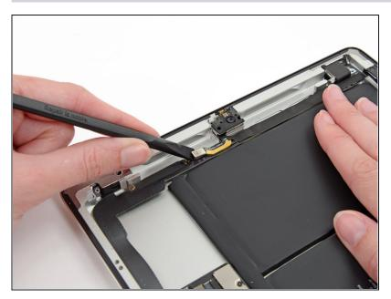
Using the flat end of a spudger, pry the front-facing camera off its socket on the headphone jack assembly.
