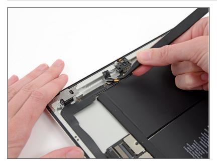
Use a pair of tweezers to peel back the adhesive tape covering the front-facing camera connector.
