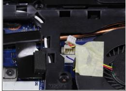
Unplug the fan power cable by pulling the cable towards you using a spudger to help pop off the connection.
