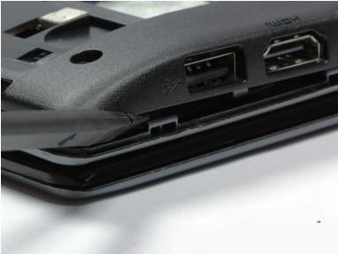
Unclip the bottom half of the case from the laptop by using a spudger and starting at the USB port on the right side of the laptop. Then work your way clockwise around the laptop.
