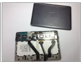
Using the plastic opening tools, continue to carefully run along the right and bottom edge, and then lift the screen from the back panel.
