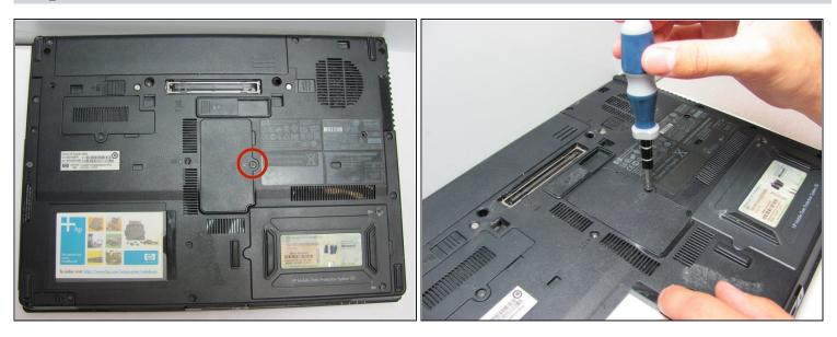
• Remove the 1.2 Philips #1 screw holding down the RAM cover to the body.
