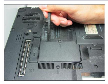
• Once the screw is removed, use a spudger to pry open the case covering the RAM chip.
