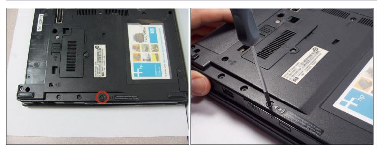
• Remove the 4 mm P0 Phillips-head screw indicated by the icon of a lock and disk.
