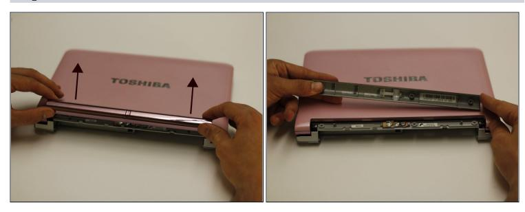
• Carefully lift off the power bar assembly for access to the button and receiver.
