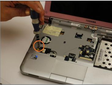
• Remove the two noted screws, 5 mm in length, with a bit driver and Phillips 3/16" tool.
