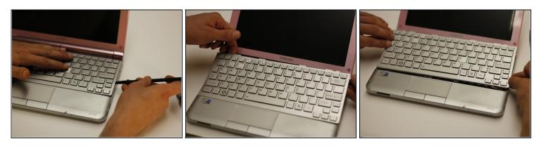
• Use the spudger to gently pry around the seam of the keyboard. This will release the keyboard assembly from the body.
