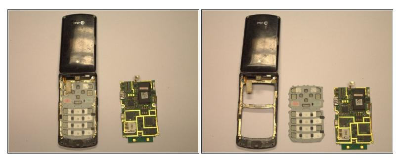
• Once the motherboard is removed, nothing else holds the keypad in place. It can easily be lifted from the phone casing.
