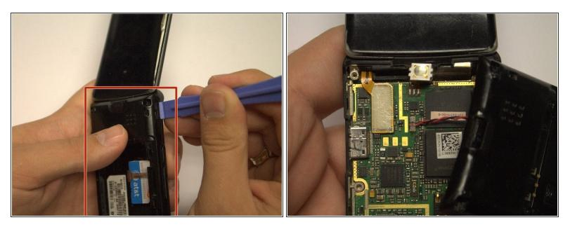
Using a pry bar or flat headed screw driver, pry the back cover from the front and lowly lift apart.
