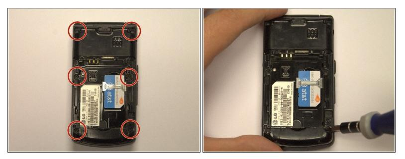
• Use a small Phillips head screwdriver to remove the six 3mm screws identified in the photo.
