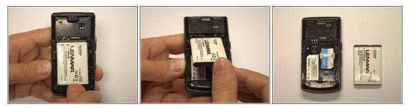
• Holding the phone in one hand and using your index finger on your other hand, remove the battery from the phone by prying it out at indention located at the bottom of the phone.
