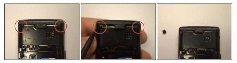
Using a spudger or other sharp tool, remove the two rubber pieces on the top of the back of the phone.
