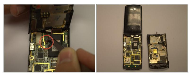
• Use tweezers to carefully unplug the wires connecting the speakers to the mother board.
