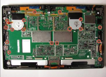
• Unscrew the 17 T5 torx screws on the mother board with the T5 torx screw driver
