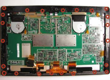
• Using a T3 Torx screwdriver, remove a total of 23 screws from the screen bezel of the Surface Pro.
