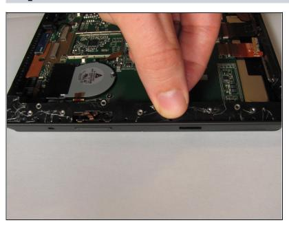
• Lift both metal panels from the frame.
