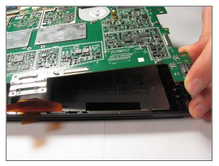
Once all screws are removed, gently lift up the logic board with your hands to pull it out.
