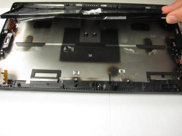
• Use your hands to pry off the entire battery pack with enough force to overcome the glue keeping the batteries in place.
