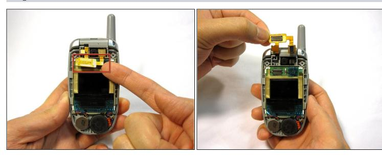
Lift the copper ribbon cable up from the bottom right hand corner.
