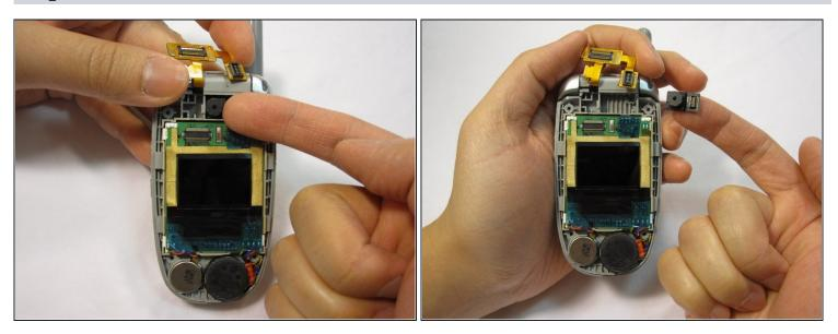
• While holding the copper connection out of the way, use your fingernail to pry the camera out of its socket.
