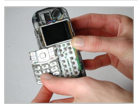
The faceplate and keypad can now be completely removed from the phone.
