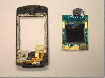
• The circuit board containing the outside and inside LCD screen should now easily remove from the phone's casing using your fingers.
