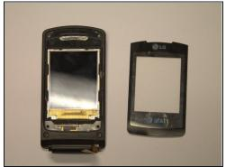
Carefully pry around the crevice of the entire plastic screen covering using a pry bar or some other type of sharp tool.
