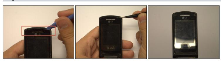
• Locate the rubber strip found above the main screen. Use the pry bar to remove the rubber strip. This exposes the screws in the upper left and right hand corner.
