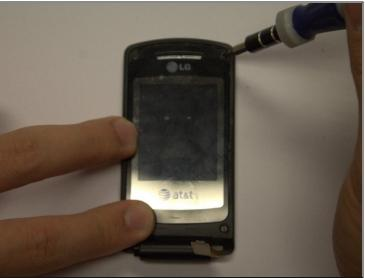
Use the small Phillips-head screwdriver to remove four 3mm screws exposed during steps 1 and 2.
