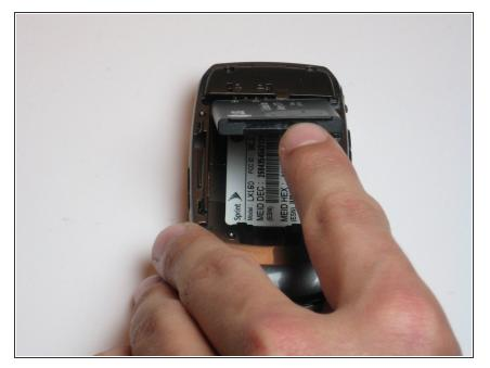
Once the panel is removed, you will see the battery. Remove the battery by sliding your finger into the notch where the LG logo was on the panel and lift the battery.
