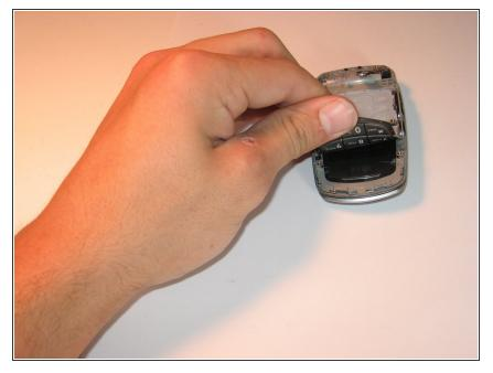
• Peel out the keypad in the back of the phone. It is the white flimsy plastic from the bottom.
