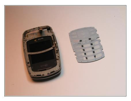
The keyboard will be separated and may be replaced with a new keyboard.
