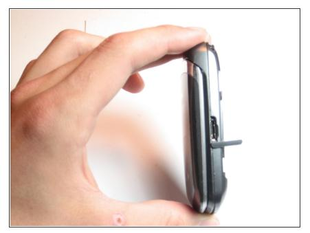
Before continuing pull off all the rubber tabs to the headphones, and the power input.
