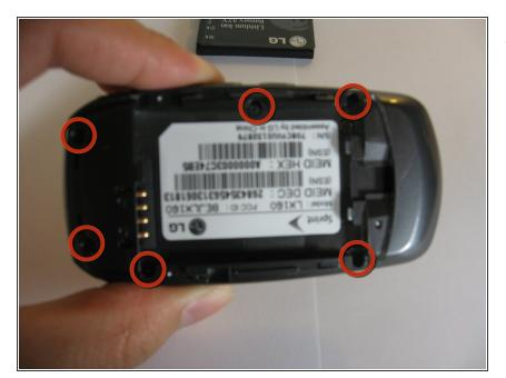
Now turn the phone so that you can see the back where the battery was. Using a screw driver, unscrew the 6 screws holding the back casing together.
