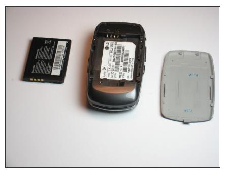
• Remove the battery completely from the phone and place the battery off to the side.
