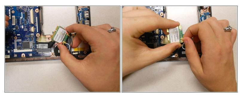
Disconnect the wires on the WiFi card. This can be done easily by applying pressure to the connections until they pop off of the card.
