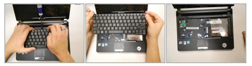
Pry up the keyboard using a spudger or plastic opening tool in the exact location shown in the photograph.
