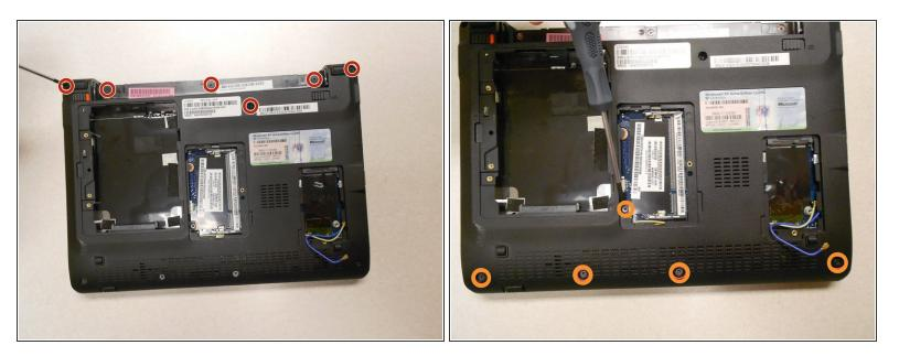
Remove six (6) 5mm screws, two (2) 17.5mm screws, and three (3) 2.5mm screws from the back, using the Phillips #0 screwdriver, as marked here.
