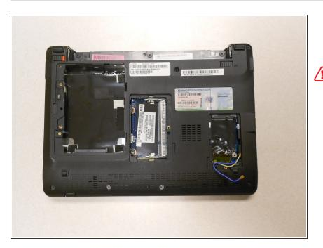
Make sure the RAM, hard drive, and WiFi card have been removed from the computer before trying to take off the cover so they are not damaged in the process.
