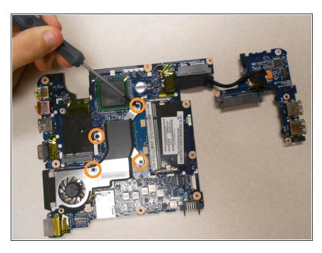
Using the #00 Phillips head screwdriver, remove all four (4) screws marked here.
