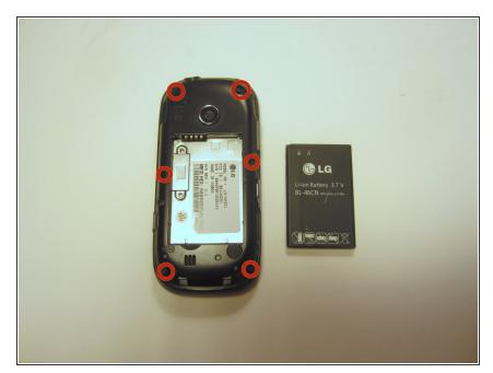
Use a screwdriver and corresponding bit to remove the six 2mm screws that are located along the edge of the rear case. Set the screws aside.
