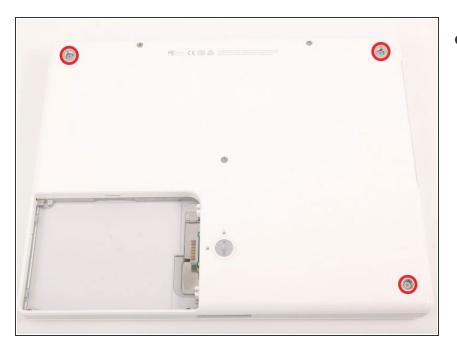
Remove the three newly-revealed Phillips screws.
