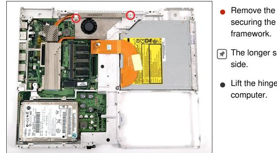
Remove the two Phillips screws securing the hinge grill to the metal
