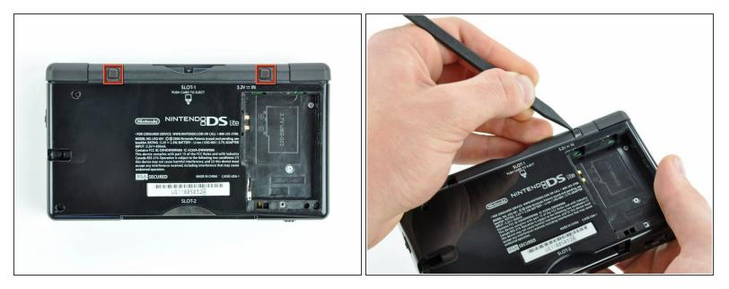
• Use the tip of a spudger to pry both rubber feet off the DS Lite.
