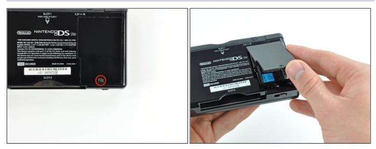
• Unscrew the Phillips screw securing the battery cover to the lower case.
