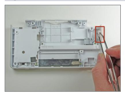
Use a pair of <u>tweezers</u> to carefully remove the power switch.
