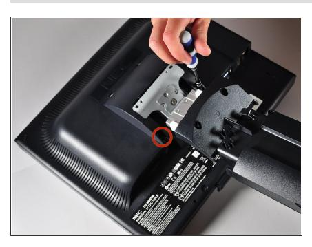
Unscrew the two 14.5mm Phillips PH2 screws holding the stand to the monitor.
