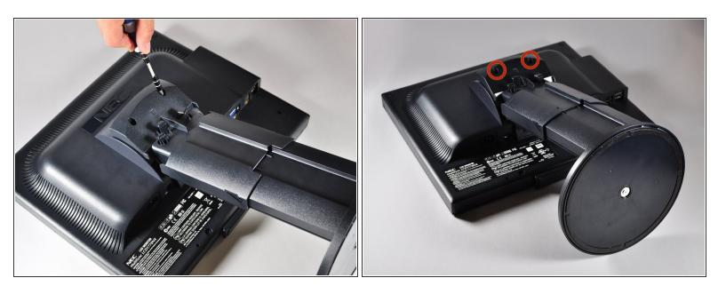
Unscrew the two 6mm Phillips PH2 screws to detach the stand enclosure from the stand.
