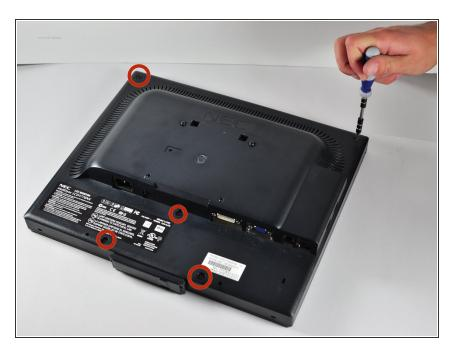
With the monitor face-down, unscrew the 5 7mm Phillips PH2 screws around the outside of the enclosure.
