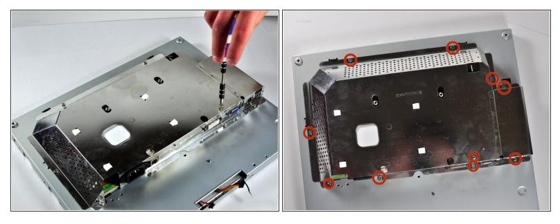
Unscrew the 10 5mm Philips PH2 screws holding the metal casing to the monitor.
