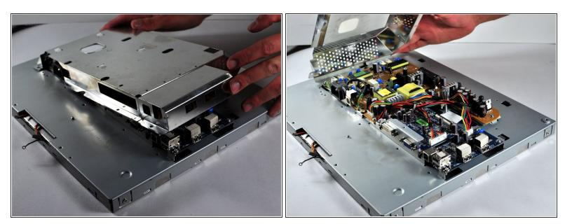
Pull the the metal casing off of the monitor to reveal the motherboards.
