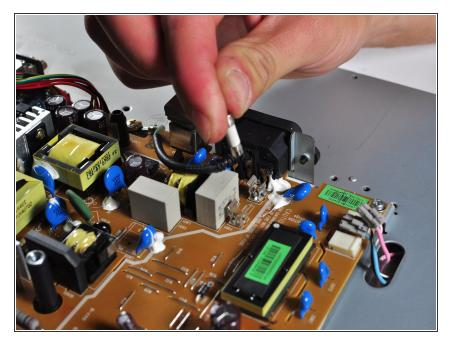
Carefully remove the power supply fuse by hand.
