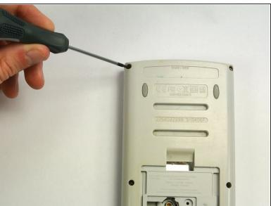
Unscrew the six 8.5 mm screws located on the perimeter of the back cover using the Precision T6
