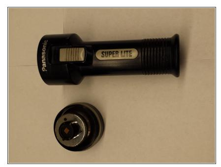
Twist the top assembly of the flashlight off by turning it counterclockwise above the rubber gasket.
