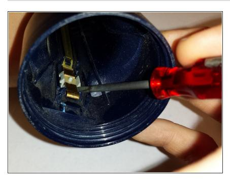
Insert the metal screwdriver as pictured: oriented vertically, underneath the yellow plastic piece
