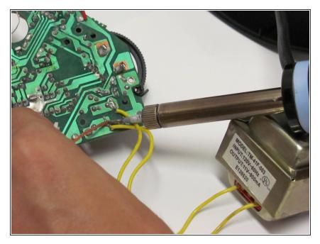
Remove the solder connecting the two yellow wires to the green quarter-circle board.
