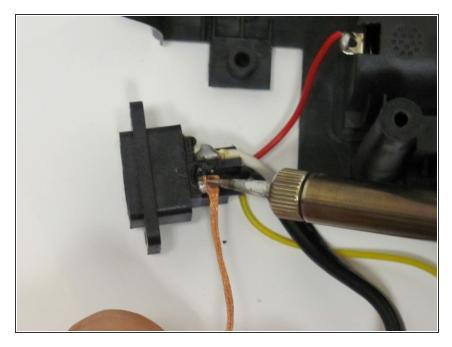
• Remover the solder from the red and yellow wires on the converter.
