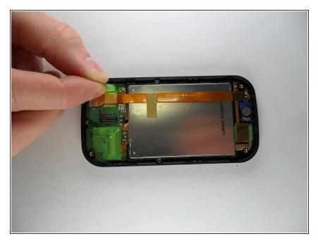
The next step is peeling off the three pieces of tape. The first two are green and located at the bottom left and bottom right of the phone.
