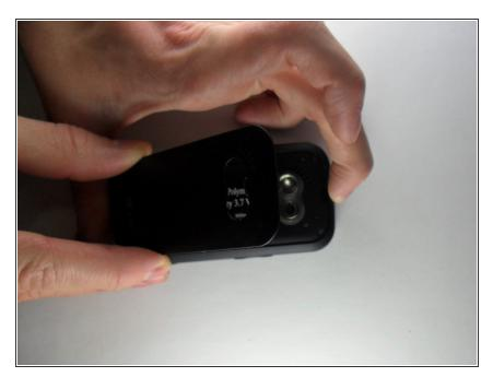
With one hand, push the rectangular button located on the back top-side of the phone.
