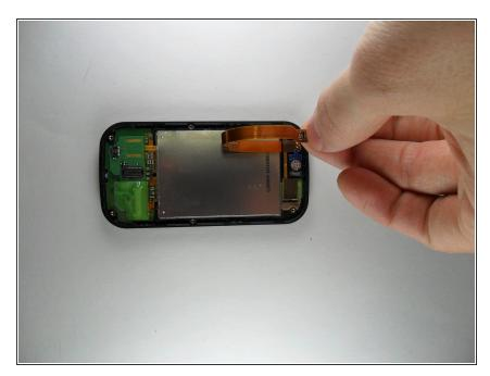
Now you need to disconnect that copper colored ribbon. it is connected at the bottom of the phone like the other ribbon. Just pop it off there. It is still attached at the top and that is ok.
