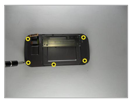
Remove 6 black screws around the edge of the slide spring frame, 1 in each corner, and 1 on each side. A screw may be covered by the slide spring. Simply move the slide spring to the other side to access that screw.
