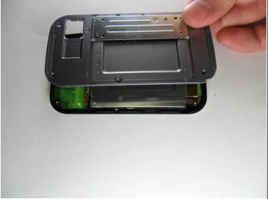
• Use the popping tool to go around the seem and slowly pull off slide spring assembly, making sure the ribbon connector does not get caught.
