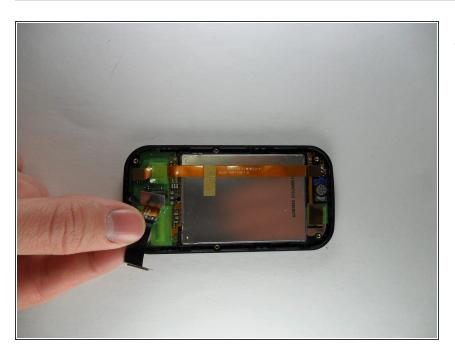
Once you have removed the slide panel and can see the back of the screen you first need to remove the connector ribbon, it is attached near the bottom of the phone. Just like disconnecting the first end of it this end is also removed by popping it off.
