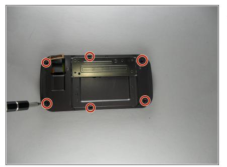
Use the appropriate screw driver head and remove the six black screws as shown in the picture. A screw may be covered by the slide spring. Move the slide spring to the other side to access that screw.
