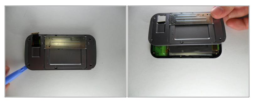
• Use the plastic opening tool to go around the seem and slowly pull off slide spring assembly.
