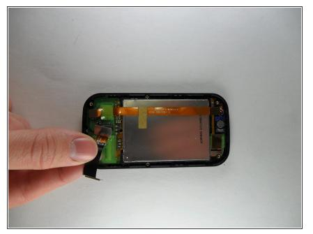
Remove the connector ribbon located near the bottom of the phone by pulling gently on the ribbon.
