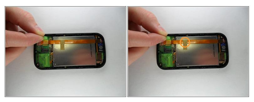
• Carefully, peel off the two green pieces of tape then the gold tape.
