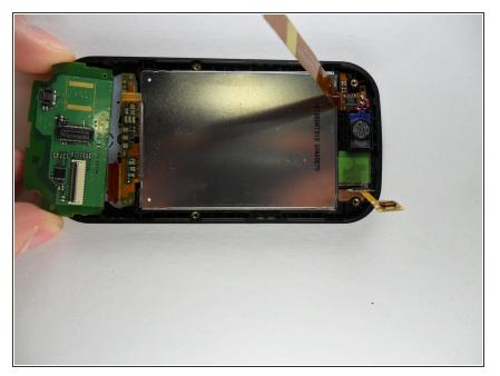
Once the silver screen has been lifted up slightly, slide the bottom half of the green circuit board located below the screen off of the phone.
