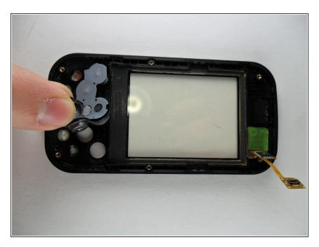
• Peel the rubber front keypad out of the case.
