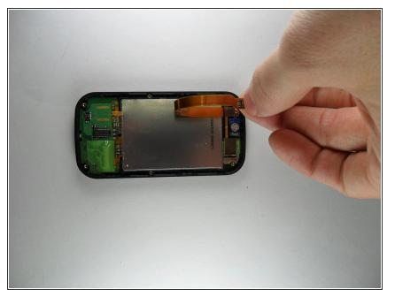
Disconnect the copper colored ribbon. It is fine to leave the copper ribbon ttached to the top of the phone.
