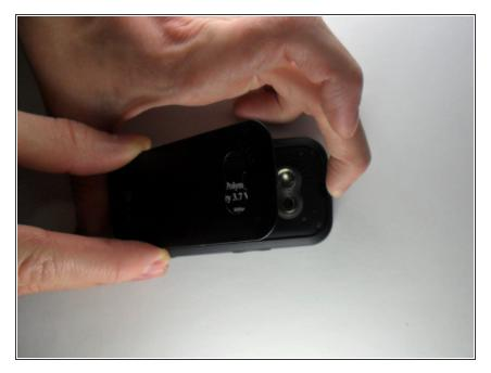
Remove the back cover of the phone by pushing the rectangular button located on the back top-side of the phone.
