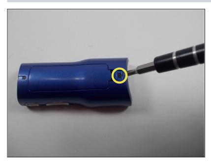
Locate and remove the screw next to the battery compartment lid.
